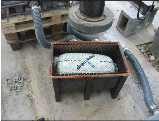
FIGURE 4: drenotube® placed on its isolated box before being tested.
