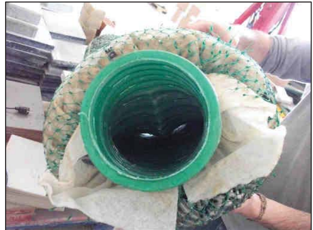
FIGURE 7: drenotube® sample 2 after drainage test under 15, 18, 21 and 24 kN axial load. Notice the strong deformation suffered by the tube, which has not been recovered once the axial load has released.
